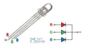
RGB LEDs have three LEDs inside them and usually, these three internal LEDs share either a common anode or a common cathode especially in a through-hole package. So basically, we can categorize RGB LEDs as either common anode or common cathode type just like in seven segment displays.
